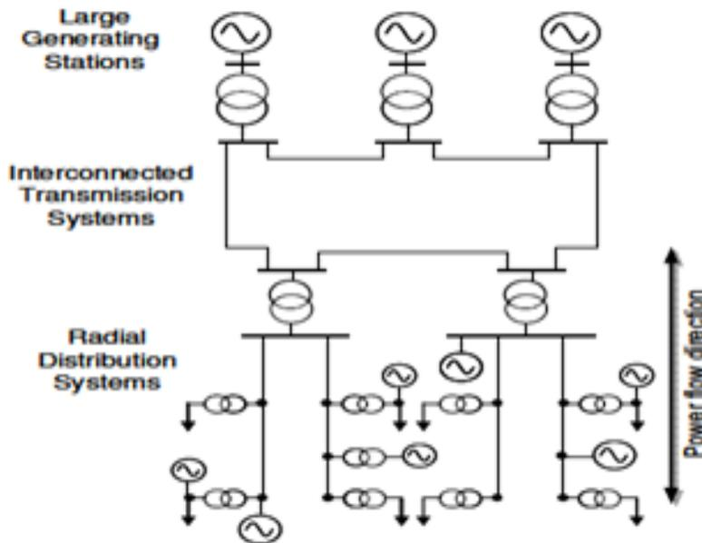
**Fig 2.4** Single line diagram of a Distributed Generation concept showing bidirectional power flow
