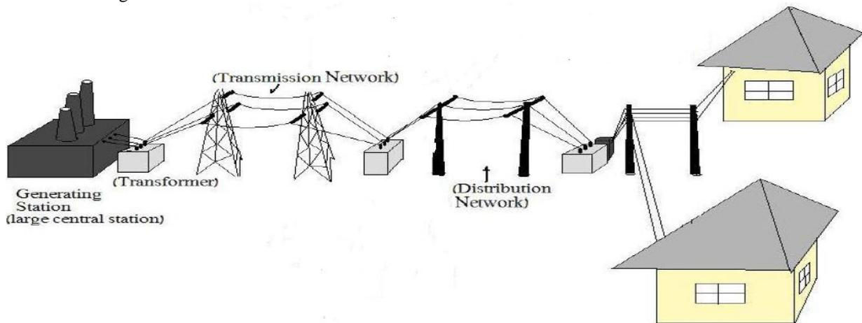
**Fig 2.1** Centralized power system showing power flows from large generating station to customer load
