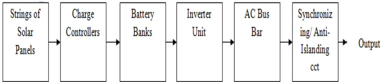
Fig 3.2 Block diagram for interfacing circuit of integrated solar panels
