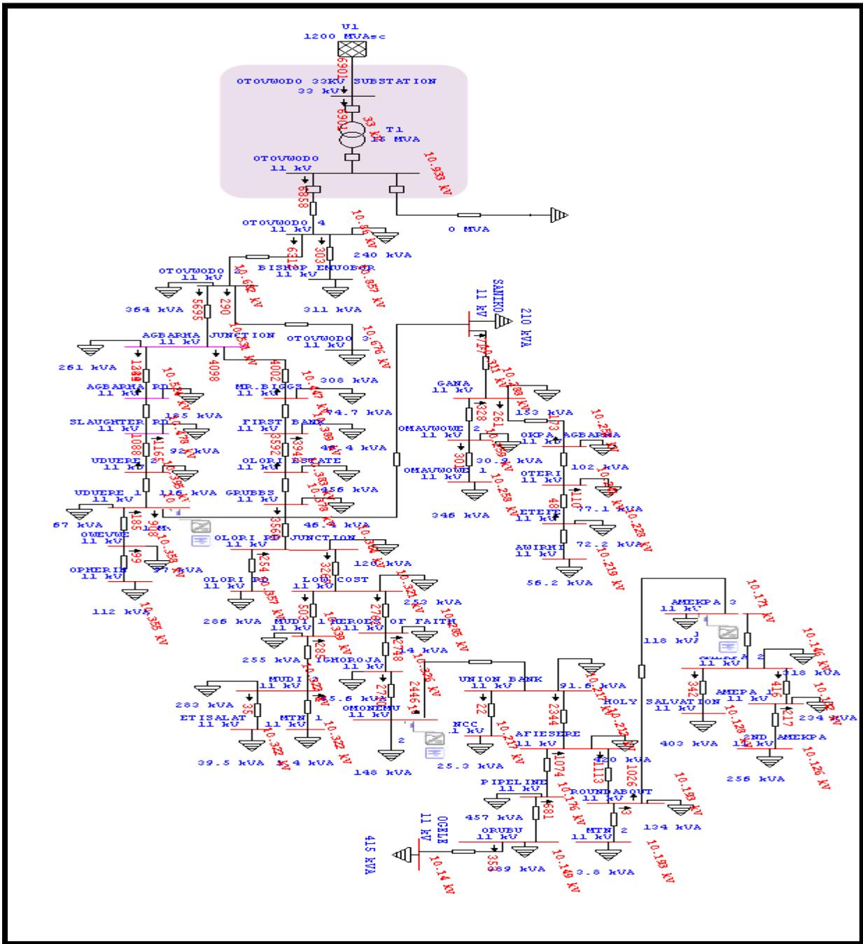
Figure 4.1: Dumez 11kV network modelled in ETAP 7.0 with Case I DG penetration
