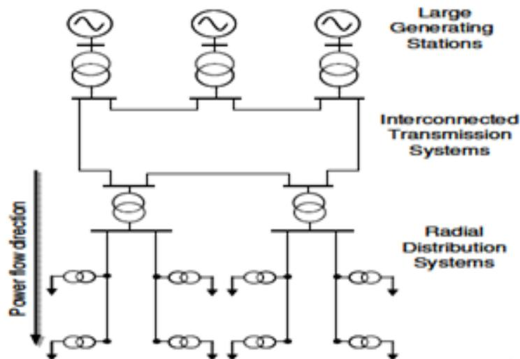
**Fig 2.2** Single Line Diagram of a Centralized Concept of Power System Nigeria
