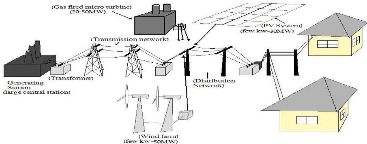
**Fig 2.3** Schematic diagram of Distributed Generation Concept.
