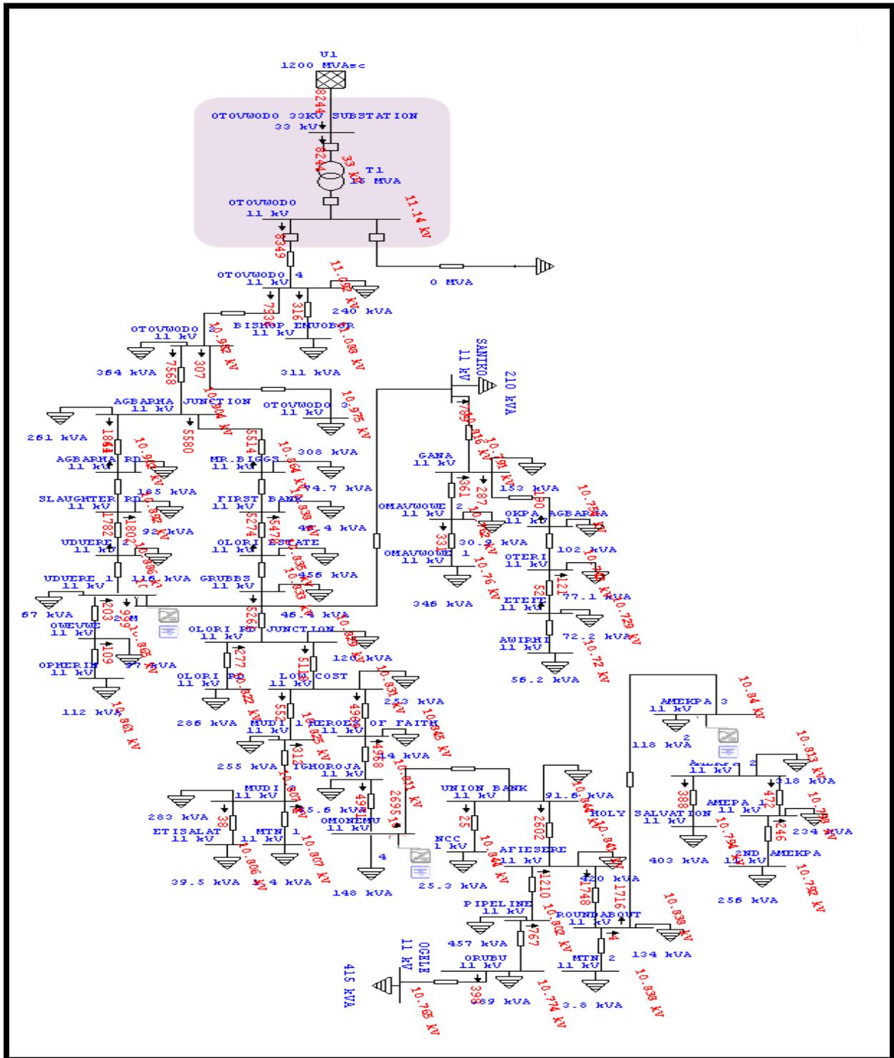
Fig 4.2: Dumez 11KV network modelled in ETAP 7.0 with Case II DG penetration
